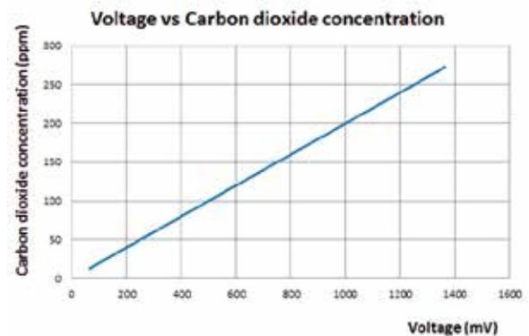
In this way the characterization of the sensor was achieved through a linear regression model, obtaining fairly accurate results. An extremely important aspect to mention is the fact that currently this issue is still being evaluated and treated, with the purpose of implementing the sensor that best shapes itself, and conditioning the signals of it with the purpose of achieving the best results.
