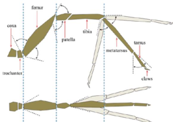
One important aspect is the amplitude that has every part of the spider leg. This means, for example, that the coxa has amplitude of 35 degrees while tibia has a mobility of 70 degrees. Also, every of the seven components of the limb, has a different axis of movement; for example, the trochanter has a movement in X-Y axis, meanwhile the femur in X-Z axis. This kind of association and motion, it's explained graphically in the figure 5.
