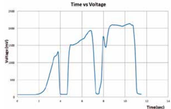
The figure 13 shows the output voltage of the sensor depending of the gas concentration reading by the sensor. In this order of ideas, a gas source was arranged next to the sensor; as the gas concentration increased, so did the voltage. Then it will show a graph that link the voltage at the output of the sensor, with the carbon dioxide concentration.
