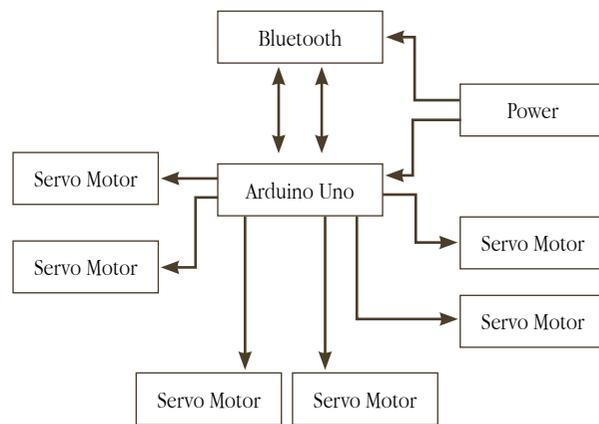
The figures 10 and 11 are representing the forward movements of each axis of the robot using Matlab ©. We use Arduino as a controller for the full platform control and communication. For motion, 12 servo-actuators were set, 3 for each leg with torque of 2.2Kg-cm. these servo-motors are attached directly as a joint of each link-leg. The supply voltage and current for the robot was a battery package of 4.8 V and 3000 mA with around power of 7.5 W approx.
